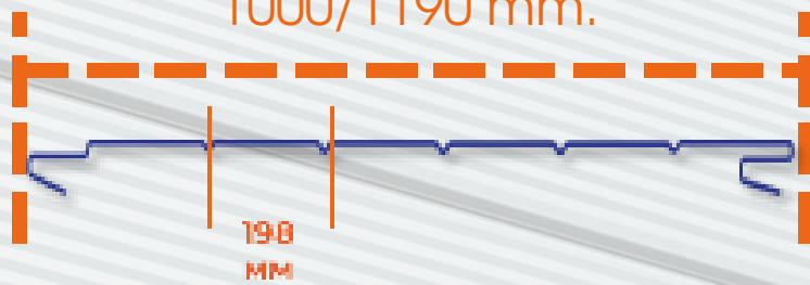
5-rib v-pitch 198 mm. 1000/1190 mm.
